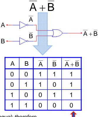
The truth-tables are equal; therefore, the Boolean equations must be equal.
