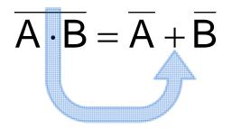
For Theorem #14A, break the line, and change the AND function to an OR function. Be sure to keep the lines over the variables.
